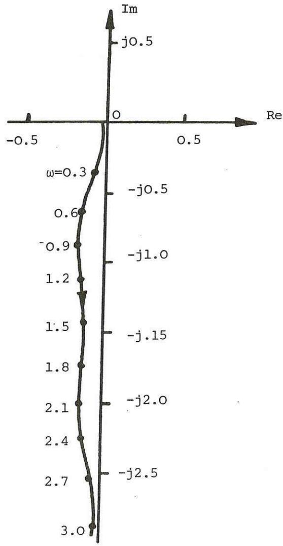
Fig. 9 Inverse Nyquist locus of  $g_2^*(o, j\omega)$  for longer column
