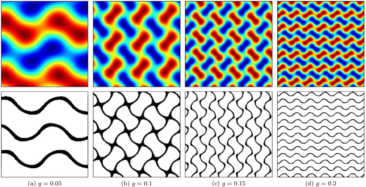
Figure 2: Vertical cross-sections through gyroids of different ‘step-size’ ( $g$ ) generated by (2), and the corresponding slices through the simulation domain after meshing the surface. Each slice consists of  $200 \times 200$  mesh elements.
