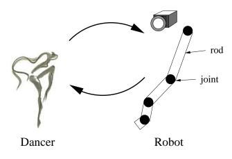
Figure 1: An overview of the SpiderCrab system showing expression flowing within a closed loop between the dancer and the robot. The robot system controls the robot, responding to the quality of the dancer's movement by biasing the robot's random movements. The dancer responds to the robot's movement.
