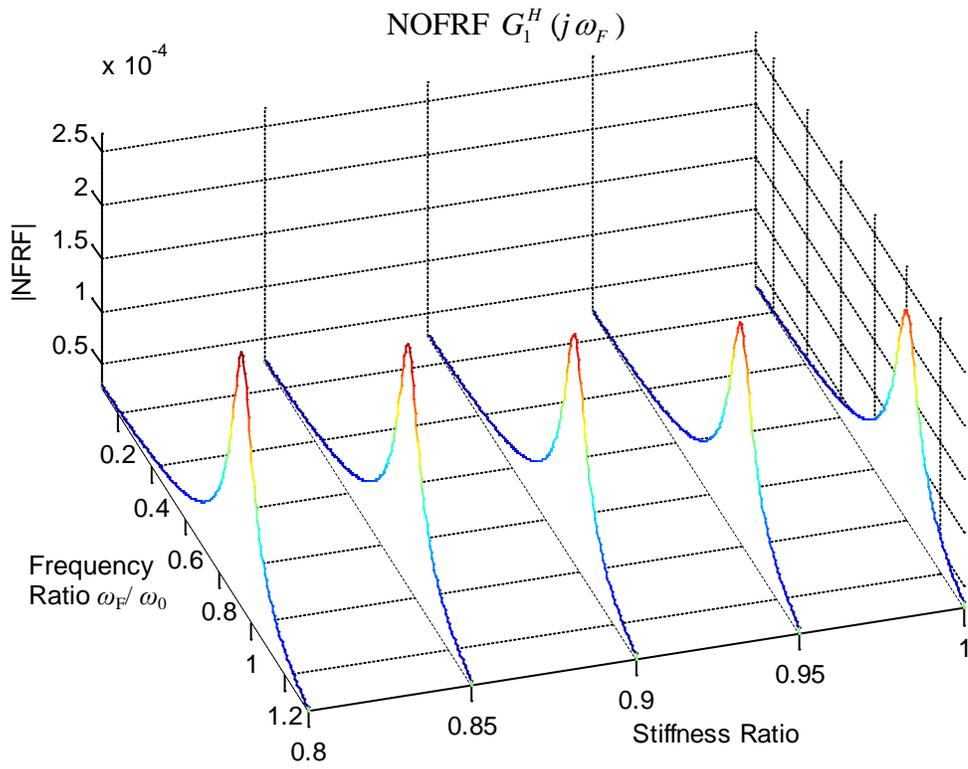
Figure 6 NOFRFs  $G_1^H(j\omega_F)$  at different stiffness ratios
