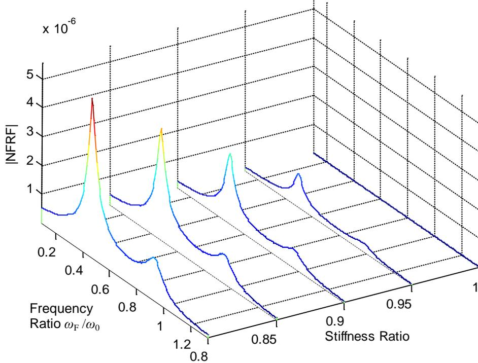
Figure 9 NOFRFs  $G_4^H(j2\omega_F)$  at different stiffness ratios
