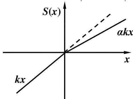
Figure 2. The restoring force of a bilinear oscillator
