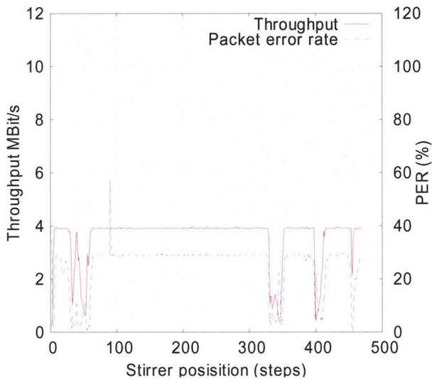
Figure 10: Wifi Packet error rate and throughput at an average Q-factor of 144
