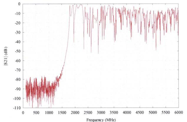
Figure 1: Coupling between two monopoles in a closed 96.5mm diameter conducting cylinder
