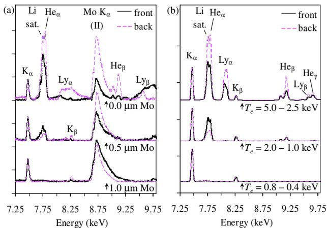
FIG. 2 (color online). (a) Experimental spectra from the front and rear side of 0.5  $\mu\text{m}$  Ni layers buried under various Mo layer depths (Mo  $\text{K}_\alpha$  in 2nd order is at 8.75 keV). (b) Modeled spectra of Ni layers at various depths with temperature and density profiles discussed in the text (Mo was not modeled).
