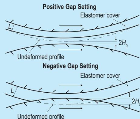
**Figure 2** Positive gap (upper) and negative gap (lower) deformable roll coating systems
