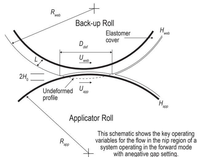
**Figure 3 Key variables in deformable roll coating**
