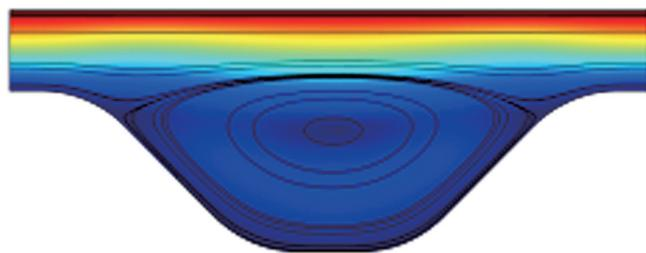
**Figure 4 Flow between the moving web and the gravure cell within the web-to-roll transfer region. The black lines show the streamlines and highlight a closed eddy within the cell, the colors indicate the magnitude of the velocity (blue = low, red = high)**
