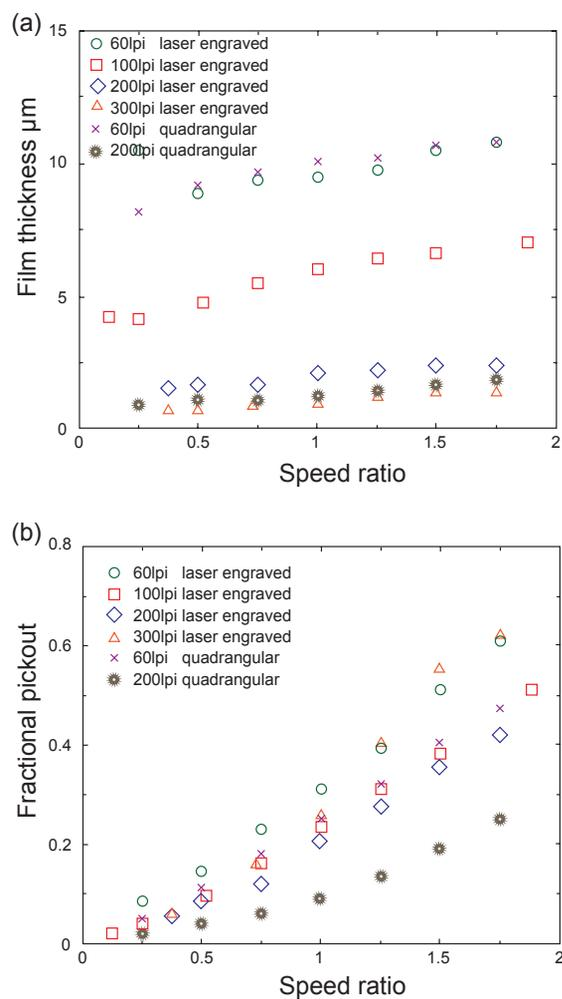
**Figure 3 Typical variation in (a) coated film thickness and (b) fractional pickout for a range of gravure rolls as the web-to-roll speed ratio is varied.**
