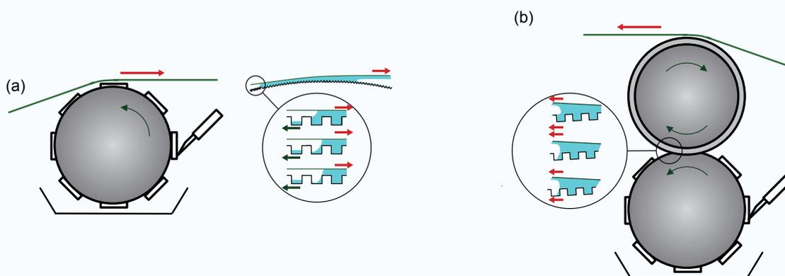
**Figure 1 (a) the direct gravure process where the gravure roll and web are in intimate contact, (b) offset gravure coating where transfer is from (i) the gravure roll to the (deformable) applicator roll and (ii) subsequently from the applicator roll to the web**
