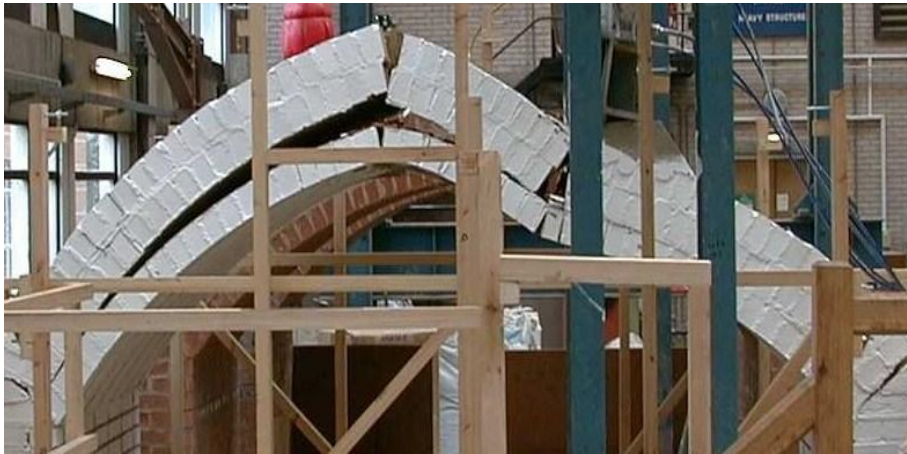
Figure 4. A reinforced arch (arch 2) without shear reinforcement showing premature partial ring separation and a 4-hinge collapse mechanism.
