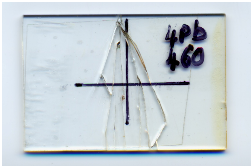
Figure A.2: Representative fracture surface of a glass specimen indented using a 1 kg Vickers load and coated twice using a 20% epoxy emulsion concentration. Fractographic observations show that fracture initiation did not originate from the indentation site, indicating effective healing of the controlled surface defect by the epoxy coating.
