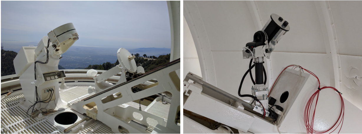
Figure 6. Left: The 60-foot Solar Tower Telescope observing platform and coelostat. Right: The automated Sky-Watcher AZ GTi Alt-Az mount and solar telescope installed on the aft-side of the second-flat pier.
