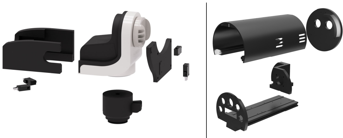
Figure 3. Left: An exploded view of a Sky-Watcher AZ GTi Alt-Az mount modified with limit switches for automatic position homing. Right: A custom solar telescope chassis supporting a solar fibre-feed, and on-board control and guiding. Not to scale.
