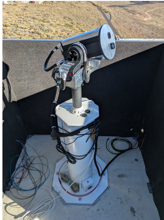
Figure 4. The automated Sky-Watcher AZ GTi Alt-Az mount and solar telescope installed on a pier inside the weather enclosure.
