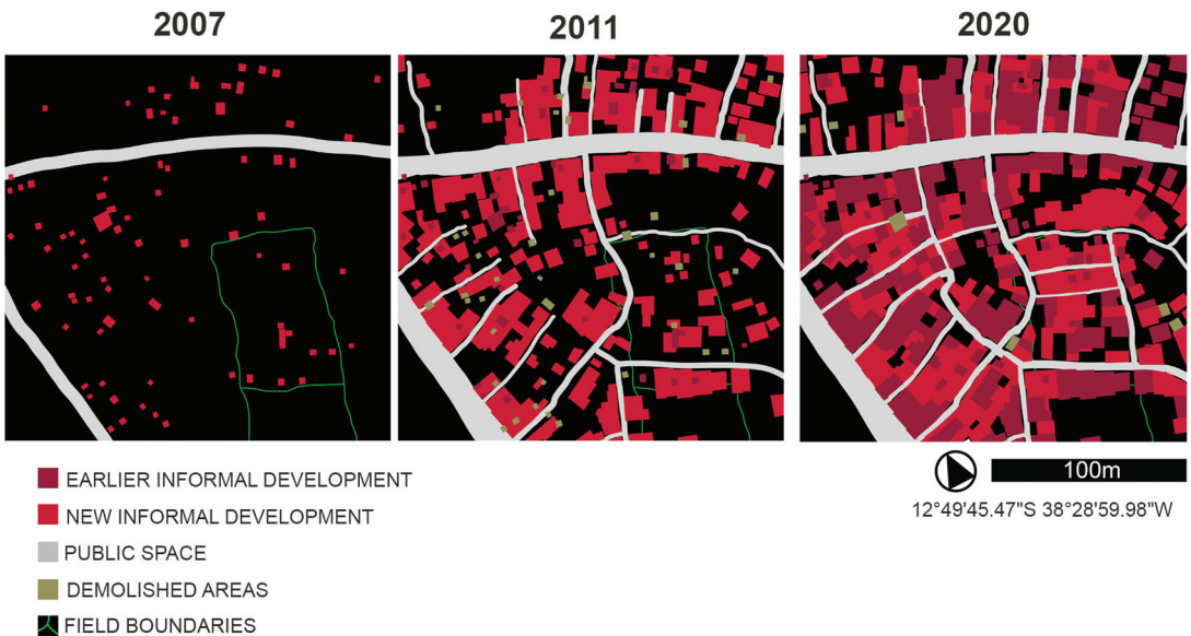
Figure 2. Iriguaçu, morphogenesis 2007–2020: incremental emergence of buildings and street/lane network. Source: Dovey et al. (2023), based on Google Earth imagery.
