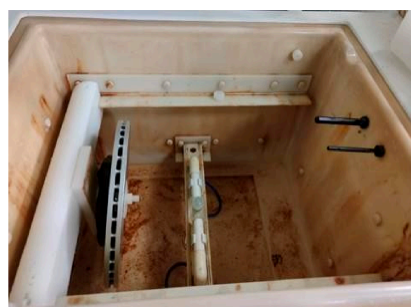
Figure 6. Salt spray chamber showing brake rotor held at 15 degrees to vertical.
