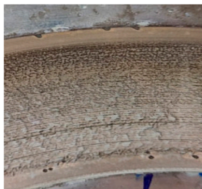
Figure 11. Enlarged image of corroded PEO rotor showing defects near inner edge of friction ring.
