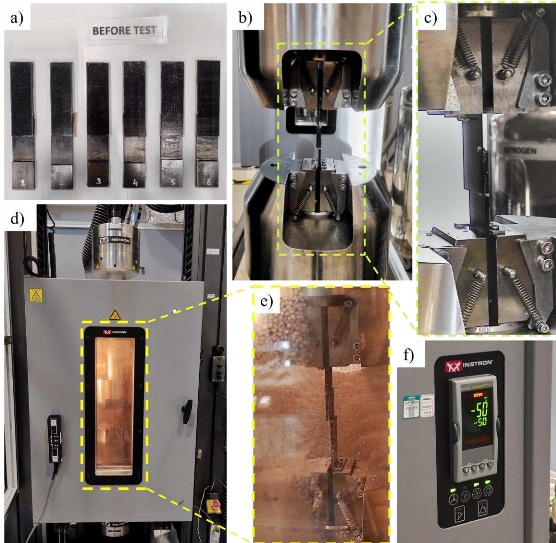
Figure 5. The single-lap shear test: a) some samples before the test; b-c) SLS fixture; d-e) the sample inside the environmental conditioning chamber; f) the temperature monitoring of the chamber.
