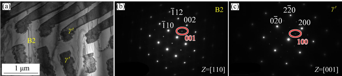
Fig. 2 TEM images of as-cast Ni35 alloy: (a) Bright-field TEM micrograph; (b) Selected area electron diffraction pattern of B2 phase; (c) Selected area electron diffraction pattern of FCC \gamma' phase
