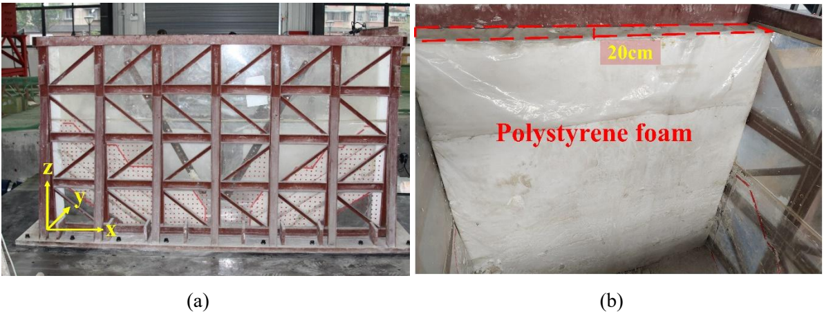
Figure 4 The model container and the measures of reducing boundary effect. (a) the model container; (b) the measures of reducing boundary effect.
