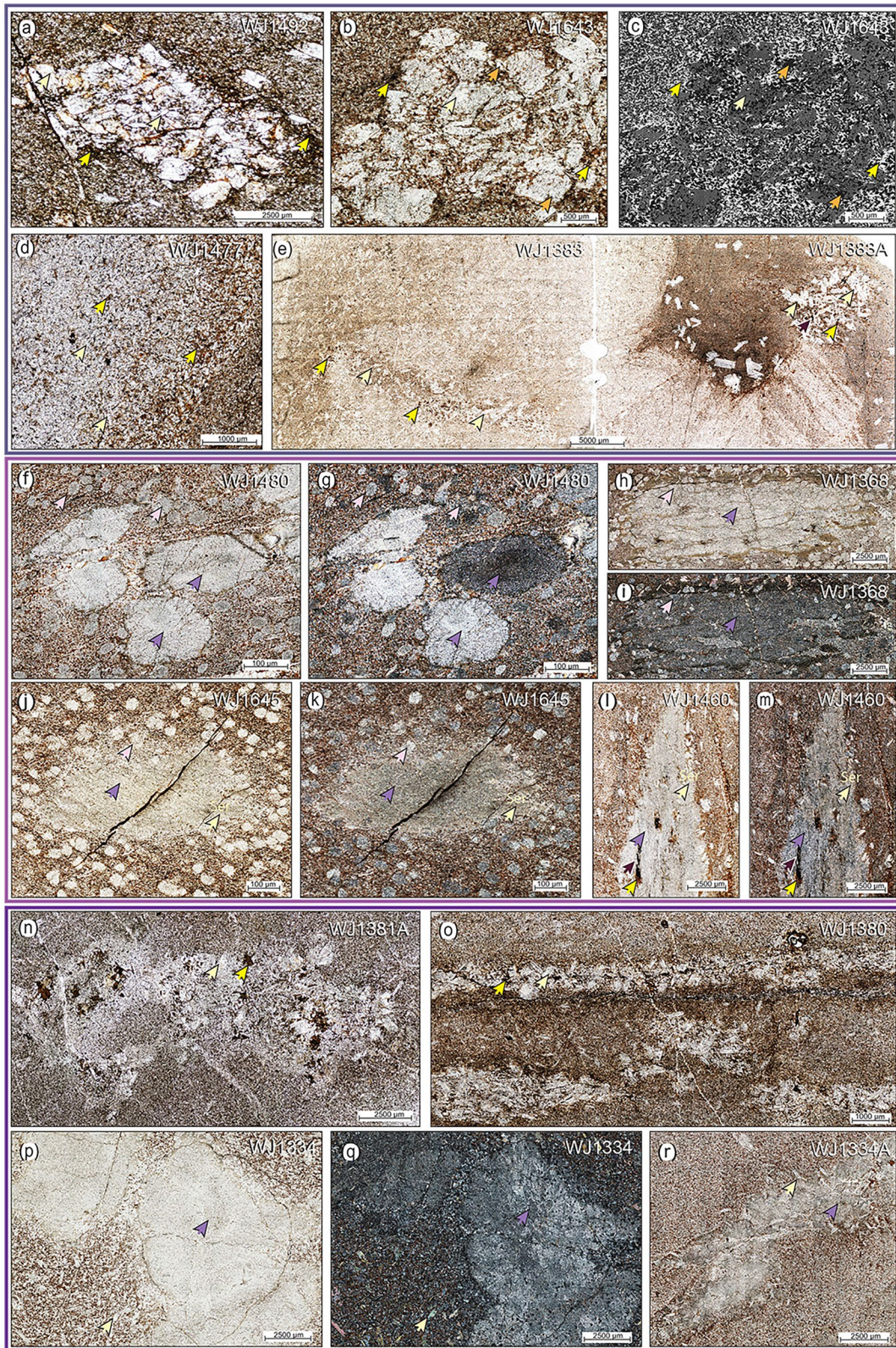
Figure 3. Clumped muscovite and cordierite. (a–c) PPL and BSE images of clumped muscovite from Unit 3 showing smaller muscovite crystals surrounded by larger ones. There is a slight increase in biotite around the clumps and some increase in quartz apparent in the BSE image (c). (d) Fine muscovite with minor biotite formed from retrogressed cordierite from Unit 3. (e) Another example of retrogressed cordierite from Unit 3 with coarse biotite in muscovite clumps. Also evident are both rounded and elongated retrogressed cordierite in the same plane (WJ1383 and 1383 A are adjoining samples). (f–g) Rounded cordierites from Unit 4. (h–i) Elongated cordierite from Unit 4. (j–k) Partly sericitised cordierite. (l–m) Strongly sericitised cordierite WJ1460. (n) Typical cordierite retrogression Unit 5a, large crystals of muscovite and large clumps of biotite. (o) Replacement vein-like cordierite retrogressed to muscovite and biotite. (p–q) Rounded cordierite Unit 5b. (r) Moderately elongated cordierite Unit 5b. Arrow colours as per Figure 2 with the addition of dark maroon, ilmenite. Sample numbers on each figure. Coloured box outlines: lavender, Unit 3; dark pink, Unit 4; purple, Unit 5.
