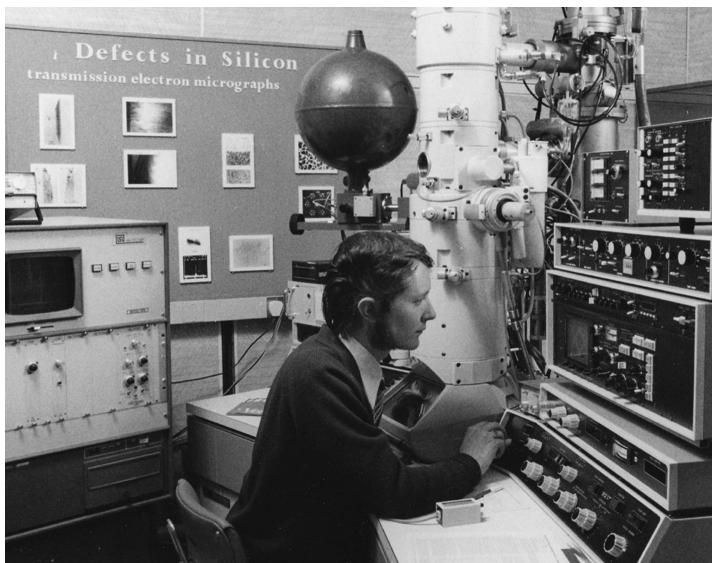
Figure 3. Tony operating a JEOL JEM 200CX scanning transmission electron microscope. (From the Cullis family collection.)
