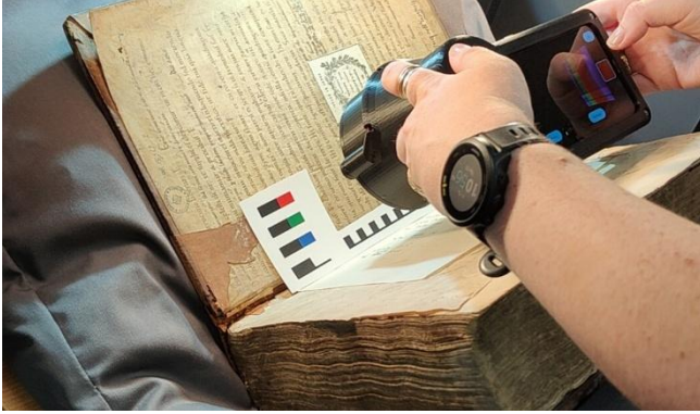
Figure 2. A spatial reference card is placed onto a sample that cannot be scanned on a translation stage due to its size and the restriction on the opening angle.
