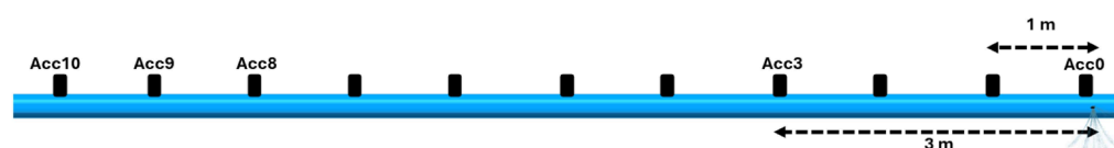
Figure 2. A schematic view of the pipe with the sensor locations.
