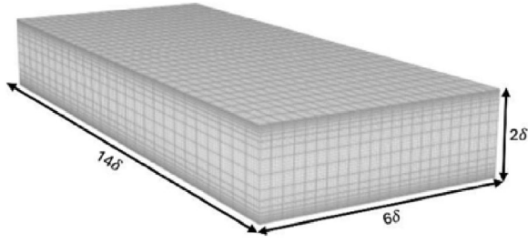
FIGURE 1 | Computational mesh demonstrating element spacings and increased near-wall nodal density. The size of the domain is specified in terms of the characteristic length scale \delta = 0.02 m, the half channel height.
