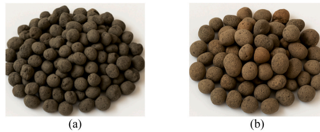
Fig. 2. Lightweight aggregate used in this study: (a) Lytag; (b) Leca.
