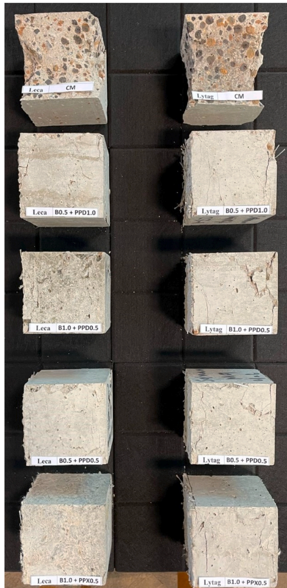
Fig. 8. Specimens after compressive strength test.
