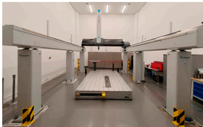
Figure 7. Hexagon DEA Delta gantry CMM setup in AMRC, University of Sheffield.
