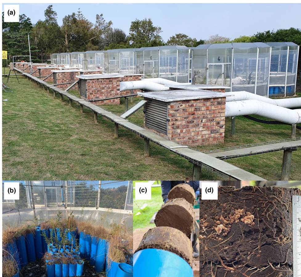
FIGURE 1 The grass-tree interaction experiment at the Rhodes University elevated CO 2 facility showing (a) Open-Top Chambers (OTCs); (b) pot culture of trees and grass in one of the OTCs; (c) collection of soil into 10-cm sections during harvest; and (d) roots and nodules of the leguminous tree Vachellia robusta .
