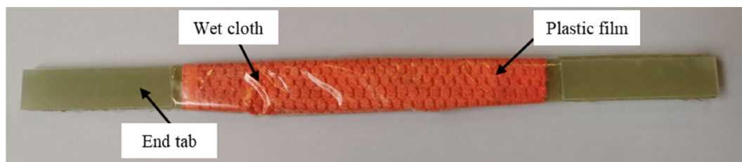
FIGURE 2 | Aged coupons were kept wet during testing by covering with a saturated cloth and plastic wrap.
