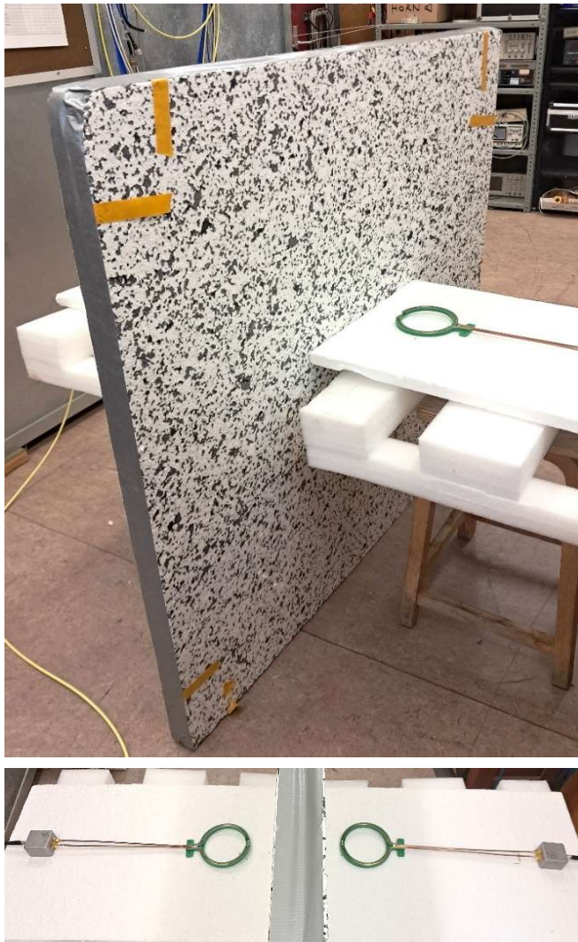
Fig. 14. Images of the SE measurement set-up for a loop to shield distance of 150 mm. The shield material veil is sandwiched between two polystyrene sheets.
