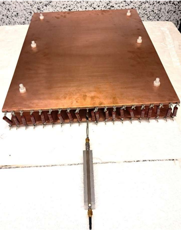
Fig. 11. The parallel plate transmission line showing the distributed matched load resistors and the field probe inserted between the plates. The parallel plate transmission line feed point is at the top of the image. The field probe balun remains outside the transmission line.
