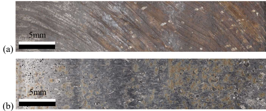
Figure 1. (a) Ground and (b) run-in railheads
