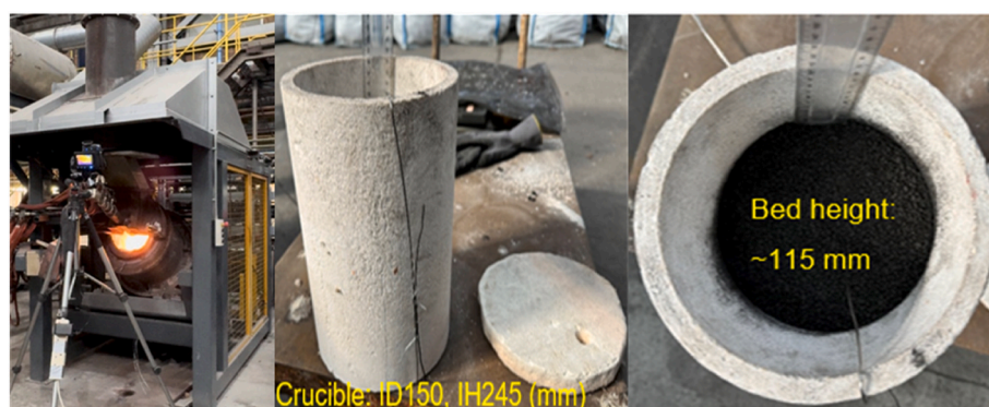
Fig. 1. Top Blown Rotary Converter (TBRC) and crucible used in the experiments.
