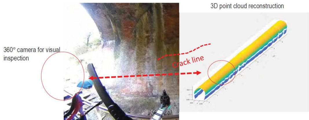
Fig. 18 Crack detection along the railway tunnels [81]
