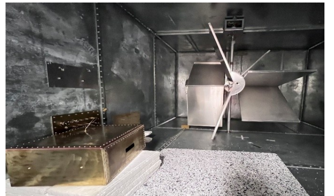
Fig. 4. University of York RC showing the enclosure with its 140\text{mm} \times 40\text{mm} aperture.
