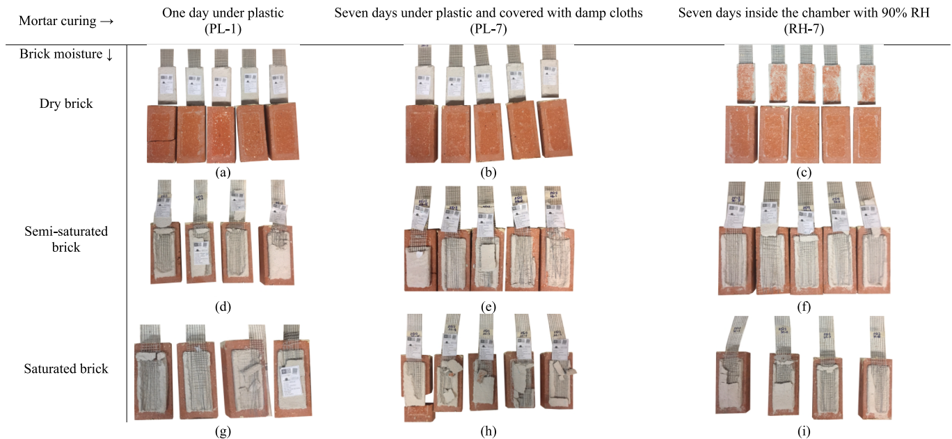
Fig. 11. Failure of the single-lap shear test samples: (a) S_PL-1_D; (b) S_PL-7_D; (c) S_RH-7_D; (d) S_PL-1_SS; (e) S_PL-7_SS; (f) S_RH-7_SS; (g) S_PL-1_SA; (h) S_PL-7_SA; (i) S_RH-7_SA.
