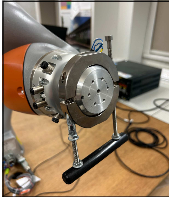
Figure 3. Modified end-effector handle with a U-shaped handle, allowing participants to easily hold and control the robot during the experimental task.
