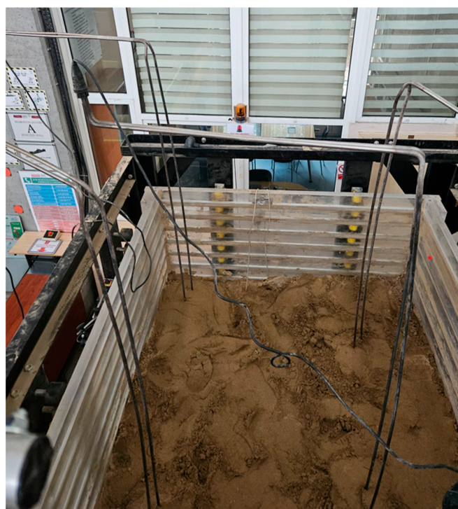
Figure 7. The drying process of the sand sample through electric rods before removal.
