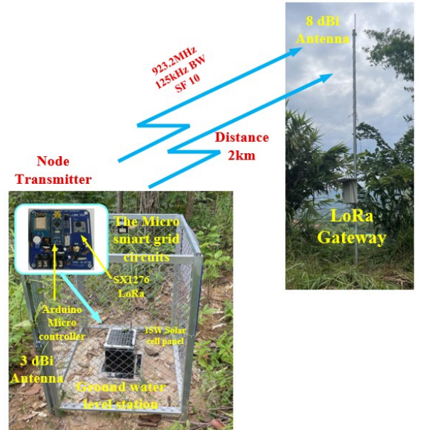
Fig. 6 The deployment of the sensor node and LoRa gateway in the real environment setup.
