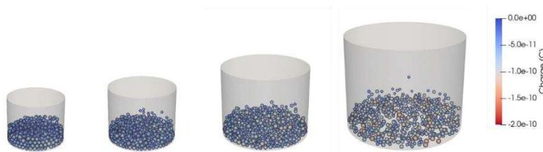
Figure 2: Snapshots of the simulated 1.5-3 mm tri-disperse polypropylene particles in the shaken glass cylinder at different volumes (25cc, 40cc, 80cc, 200cc).
