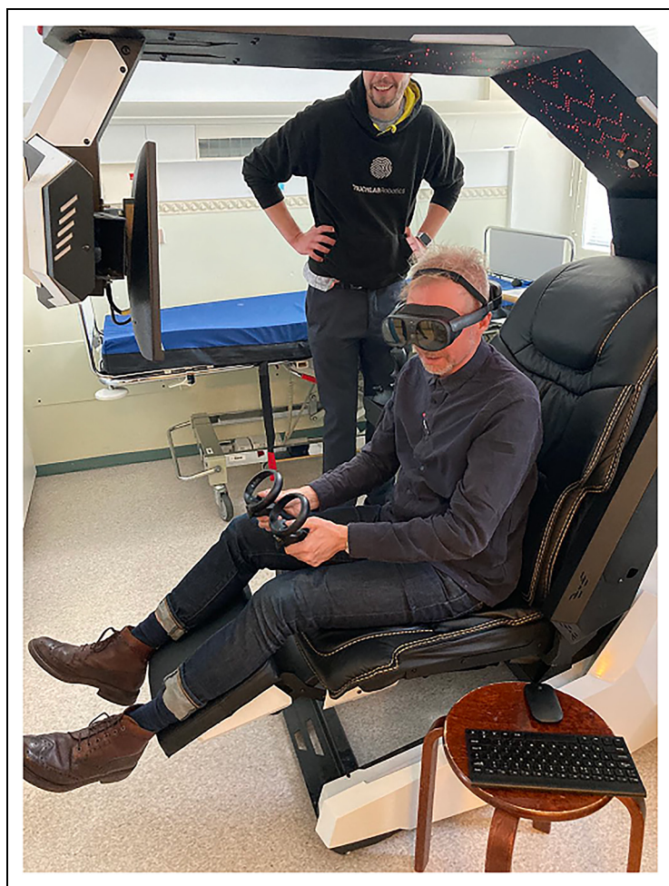
Figure 2. Teleoperator with trainer. The photo shows one of the research team members sitting in the scorpion chair using a virtual reality (VR) headset and hand controls to operate Vålky. May 27, 2023, Helsinki, Finland.
