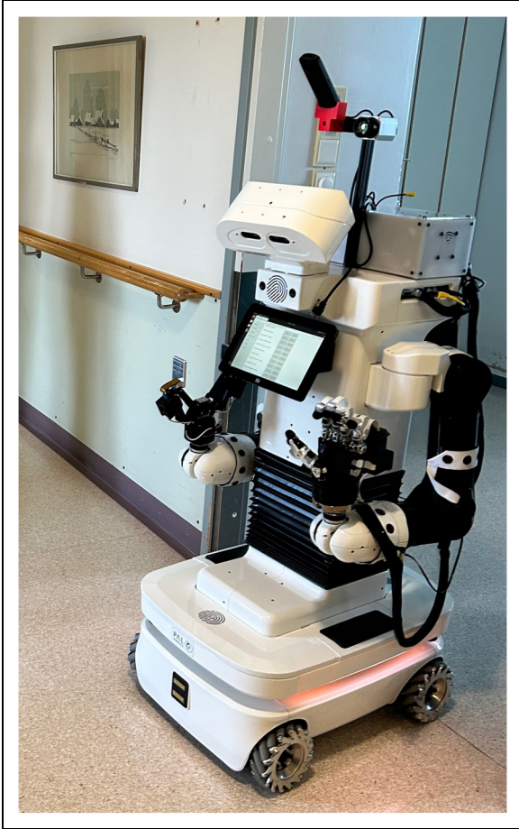
Figure 1. Vääkky robot. The photo shows Vääkky in a hospital corridor. The robot is a white PAL Robotics modified TIAGo robot. It is white, has a basic humanoid form—two arms, torso, head—on a mobile base with wheels. The robot has articulated arms, with one human-like hand, with four fingers and a thumb, and the other “hand” is a gripper tool. There is a screen display at the robot’s chest area facing outward, and a microphone and camera above the robot’s head. Image taken on May 27, 2023, Helsinki, Finland.
