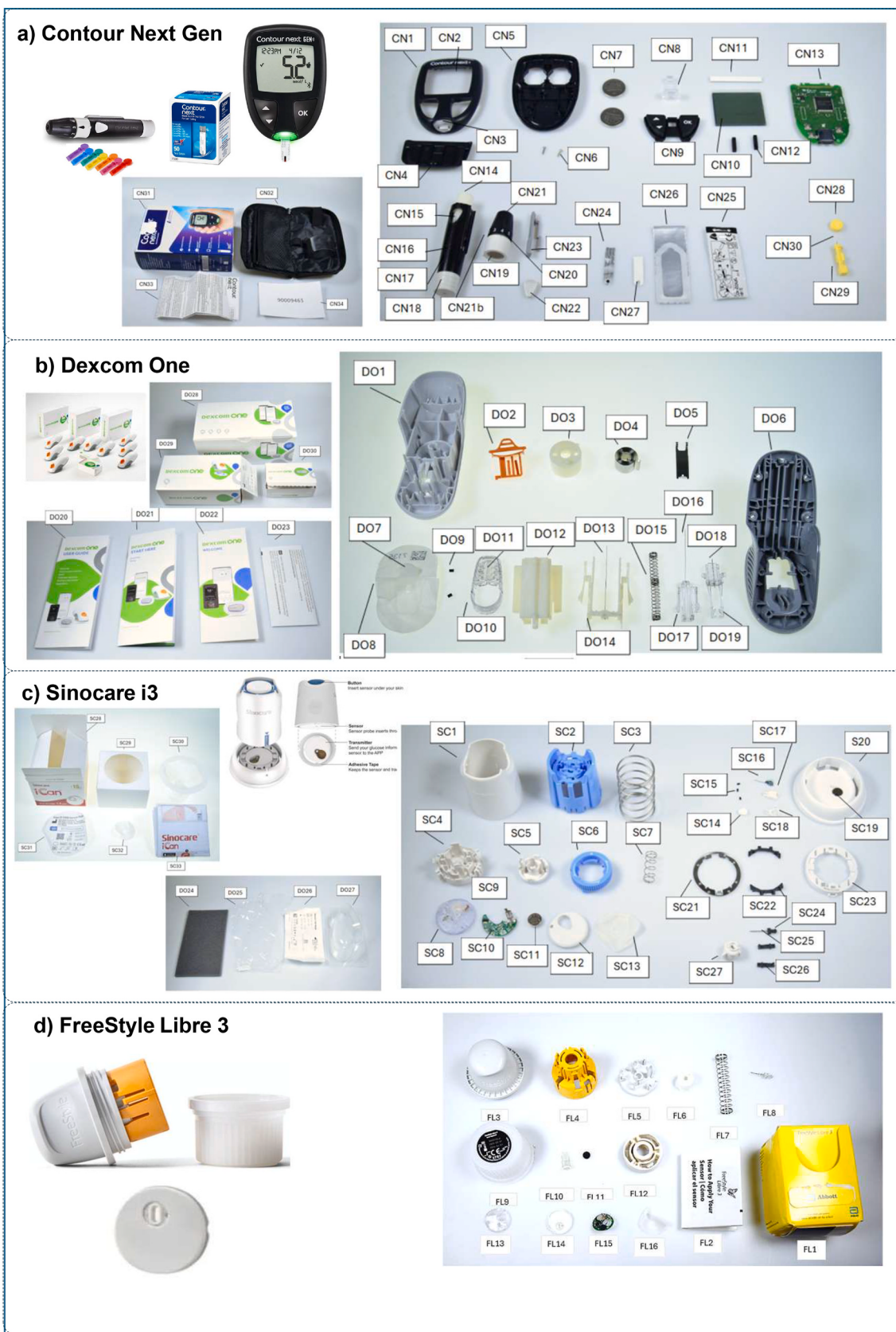
Fig. 1. The four glucose monitor systems under analysis showing the main unit, packaging and a disassembly of the component parts in a) Contour Next Gen b) Dexcom One c) Sinocare i3 and d) FreeStyle Libre 3.
