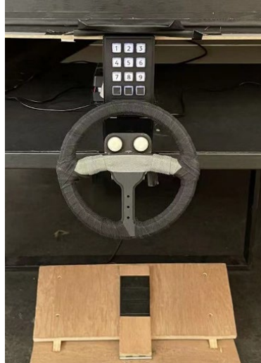
Fig. 4. The steering wheel (showing two white buttons, either of which could be used to indicate the detection of a vehicle lane change), the foot switch to indicate the detection of an obstacle and the keypad for manual responses in the number fixation task. Note: the photograph was taken with room lighting switched on.
