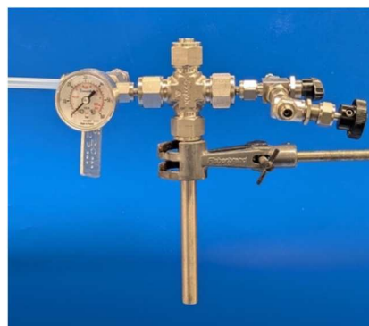
Fig. 10 Custom made pressure reactor allowing for SC-SC reactions up to 20 bar working pressure.
