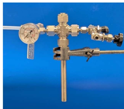
Fig. 10 Custom made pressure reactor allowing for SC–SC reactions up to 20 bar working pressure.
