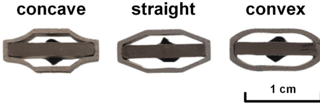
Fig. 2. Prototypes of the class IV miniature FTs incorporating concave, straight, and convex metal shells, respectively.
