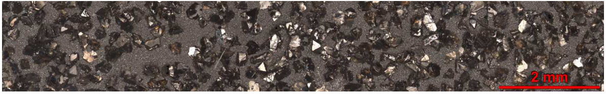
Figure 7: Portion of a blade showing the non-uniformity between grits in terms of colour and shapes.
