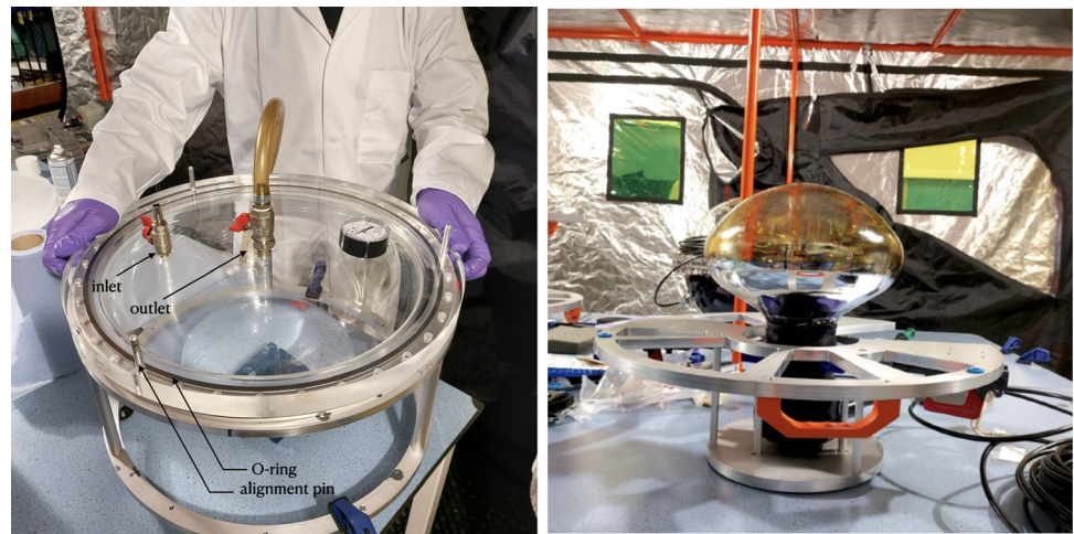
Fig. 6 Assembly process of the front hemisphere. Left: mixed RTV27905 optical gel being poured into the acrylic dome prior to degassing. Right: 10-inch PMT secured vertically in the alignment holder, ensuring correct positioning during gel curing
