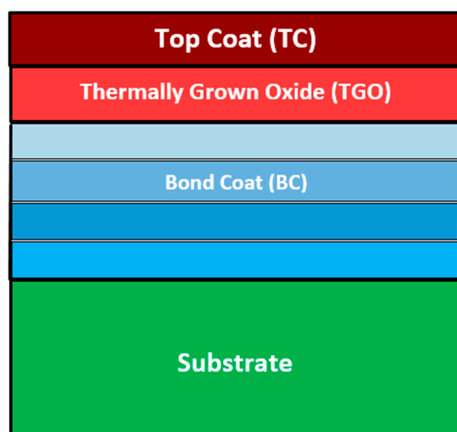
Figure 1. Schematic diagram of proposed UHTM system consisting of substrate and environmental coating (see text). The substrate would be a metallic UHTM, and the environmental coating will consist of three parts, namely a bond coat (BC), thermally grown oxide (TGO) and top coat (TC). The bond coat would be either multilayer (in the figure the BC is shown to consist of four layers), or functionally gradient material.
