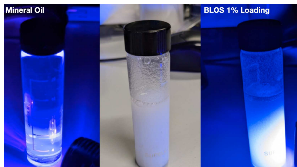
Figure 1: A vial containing an early BLOS formulation. Left: Base material under UV light. Middle: Base material with boron nitride zinc sulphide added. Right: BLOS under UV light showing light confinement within the vial.
