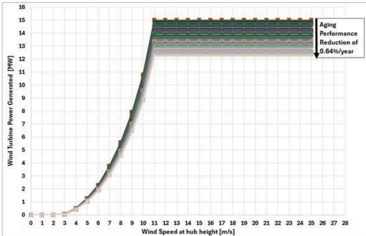
To compute the **annual Capacity Factor (CF)** for each year, the generated power (derived from the power curve) was multiplied by the expected occurrences of each wind speed value as described by the annual Weibull distributions. The CF for year  $y$  is computed using the following integral:
