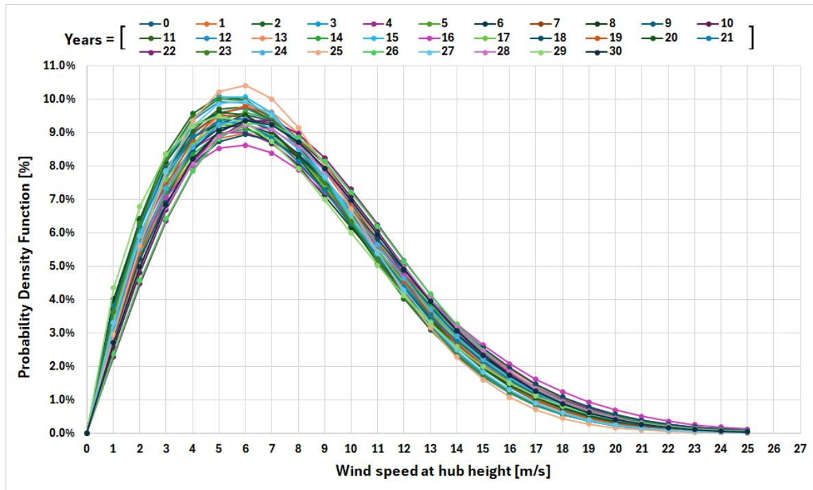
For each synthetic year, wind distributions were used to simulate the expected power production from a turbine at hub height. The turbine model selected for this study was the IEA-15-240-RWT (<https://github.com/IEAWindSystems/IEA-15-240-RWT>), which defines the expected power output as a function of wind speed at hub height. The power curve of the turbine was implemented following the methodology described in [RDS Lanni 2023], based on the following equation:
