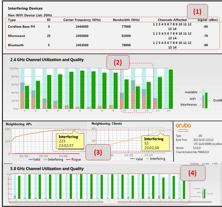
Figure 8: Level of RF interference at the experimental testing site. The radiating devices are identified in (1). In (2), the quality of the channels and their noise level are presented. The amount of neighboring APs and clients is shown in (3). Channel utilization at 5.8GHz is shown in (4).
