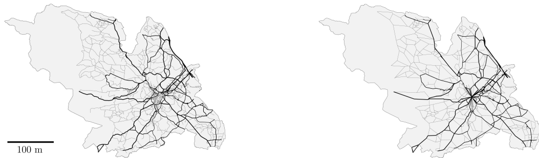
(a) Full network (3943 nodes, 8405 edges), consisting of motorways, A, B, tertiary, and unclassified roads.
