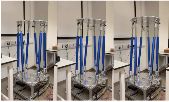
Fig. 6. Physical demonstration of the proposed PINN-PMP framework on the 6-SPS parallel manipulator.
