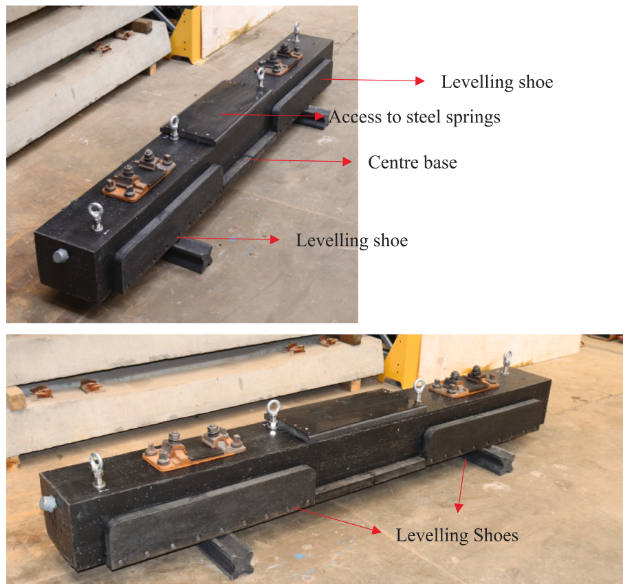
Fig. 17. Full-scale prototype of self-levelling sleeper – horizontal wedge principle (SLS-HW) .
